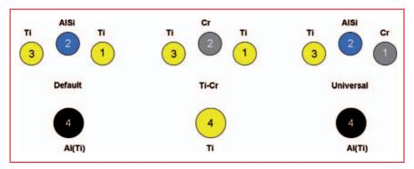
Fig. 3. Three most important cathode configurations of the  $\pi$ 313
